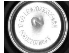
can inspection VIA-RD dome light
