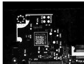
PCB board inspection VIA-LS line light
