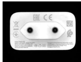
charging head detection VIA-PZRI polarized ring light
