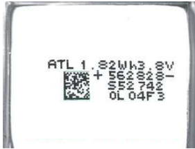
battery QR code detection VIA-CO coaxial light
