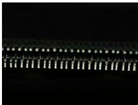
connector detection VIA-RI ring light
