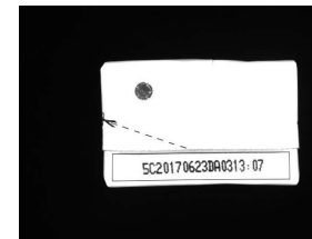
milk carton inspection VIA-CO coaxial light
